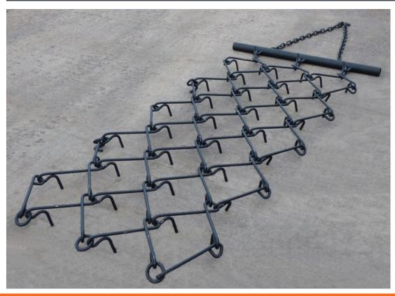
Our Superflex chain harrow section is designed to be compatible with Parmiter frames and drawbars. Manufactured from 1/2" diameter high quality carbon steel ensuring that the harrow is extremely strong with a high resistance to wear. The section is supplied in 3'-3" widths x 7'-6" depth.
