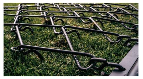
Paddock harrows are designed to cover all applications from small holdings to sports arenas and equestrian centres and are manufactured from 1/2" diameter high quality high carbon steel which ensures that the harrow is extremely strong with high resistance to wear.
