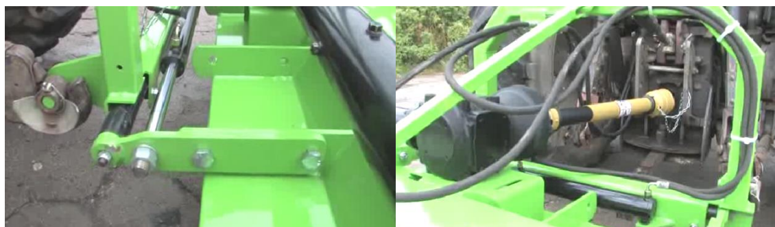
Figure 2. LEOPARD shredder – hydraulic travel of the machine
