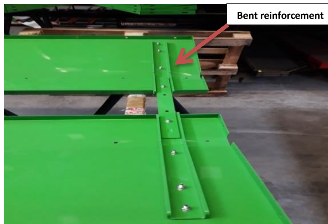
Figure 27 Step II bent reinforcement assembly
