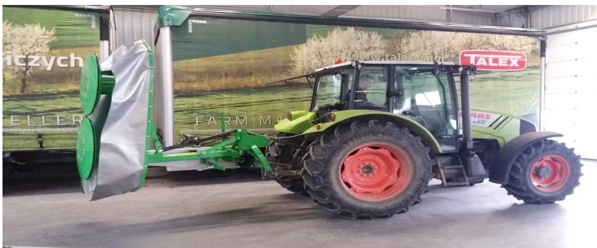
Figure 13 Proper transport position for 2.10m, 1.85m and 1.65m mowers with hydraulic cylinder
