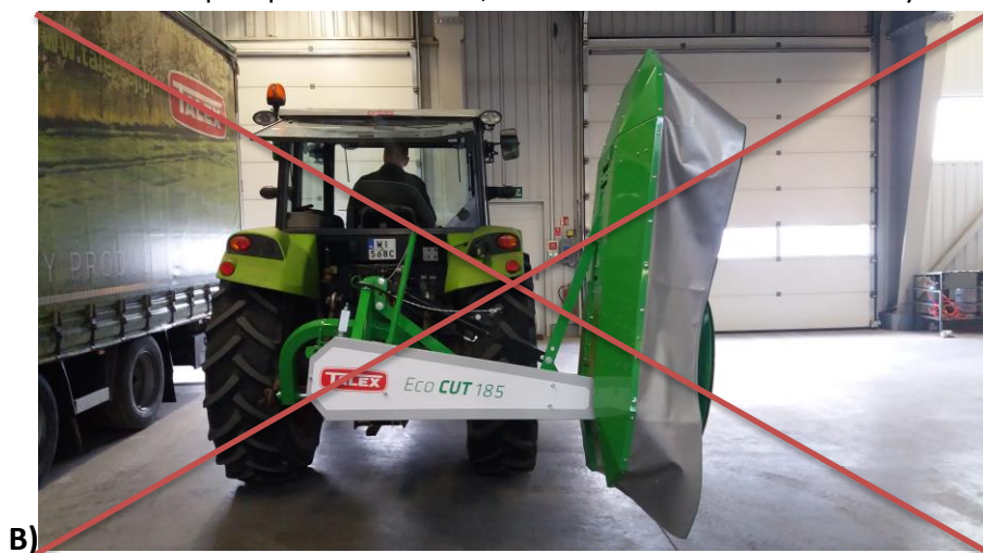
Figure 16 Incorrect transport position for 2.10, 1.85 and 1.65 mowers, models with a hydraulic cylinder (transport position width greater than allowed by law).
