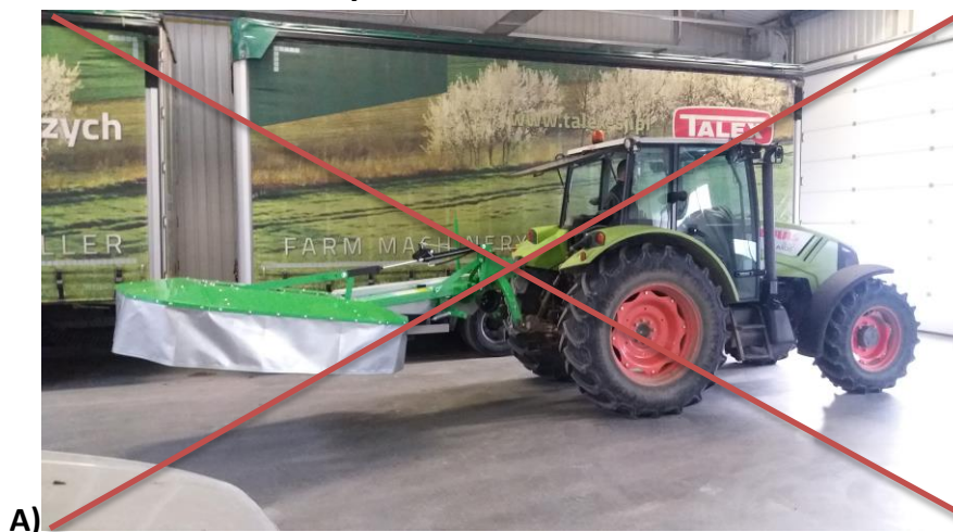
Figure 15 Incorrect transport position for 2.10, 1.85 and 1.65 mowers with a hydraulic cylinder
