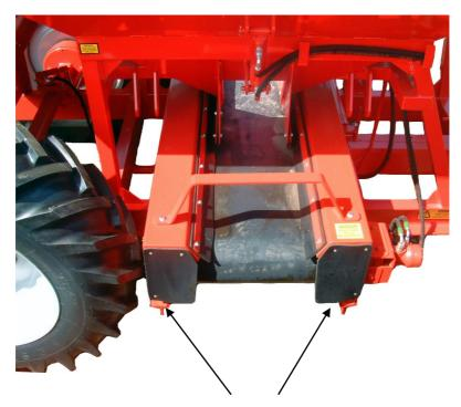
**Grease periodically (40 Hours)** 2 qty Grease Points on each end of the conveyor
