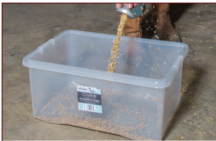
Container for gathering incremental samples
