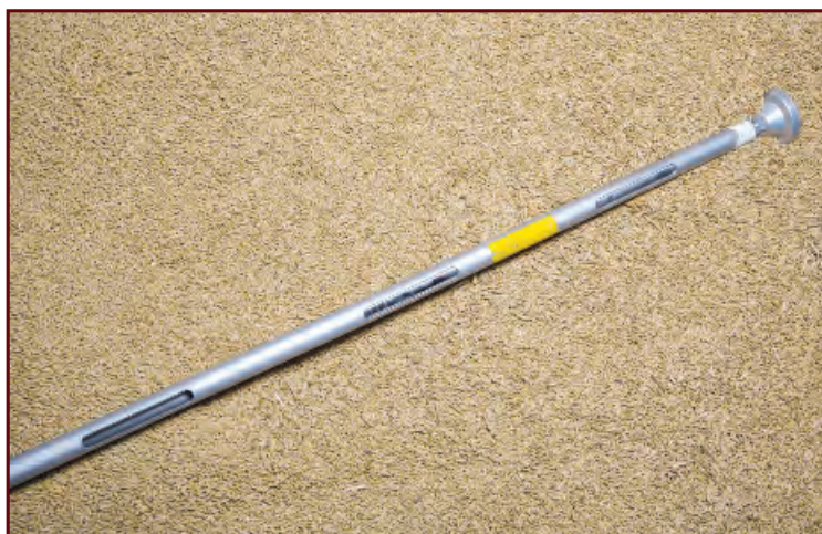
Multi-aperture sequential spear
