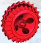
The unique Guttler self cleaning roller has two Guttler cast iron Prisma rings working together, on a 45/50 cmØ roller. The smaller ring fits snugly on the shaft whilst the larger ring runs on the inner shoulder of the smaller ring giving a cleaning action to the outer surface.
